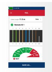
Cable test with remote attached shows remote ID number 1, length and pairing of each wire and cable performance of up to 2.5 Gb/s but failed the test due to a user-set limit of 10 Gb/s performance.
