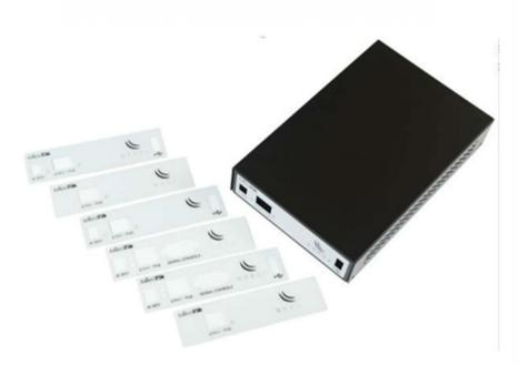
CA411-711 is new indoor case for RB411 and RB711 series. It has changeable front panels, so you can choose one that fits the product that you actually use. Also, case is higher to accommodate high-power wireless cards and has wall mounting holes on the back.
